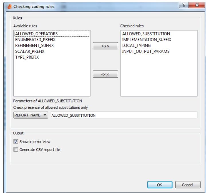
The GUI contains also two check boxes used to specify how results of coding rule checking must be shown. These results can be either displayed in the “Error” view of AtelierB main GUI, or written in an output CSV file.
